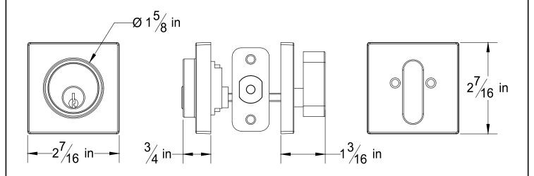
Door Prep: Cross Bore 2 1/8+, Edge Bore 1+, Mortise Latch Face 1+x 2 1/4+, Optional Drive In Latch 1" Diameter Drilled Hole
