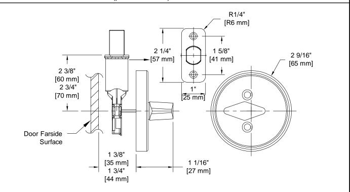
Door Prep: Cross Bore 2 1/8+, Edge Bore 1+, Mortise Latch Face 1+x 2 1/4+, Optional Drive In Latch 1" Diameter Drilled Hole Latches: Ships With Mortise Latch As Shown Above. Optional Drive In Or UL10C Fire Rated Latches Available Backset: Adjustable Latch to 2 3/8+or 2 3/4+ Door Thickness: Fit all 1 3/8+- 1 3/4+Standard Doors Strike Plate: 2 1/4+Full Lip Strike Bolt: 1+Throw
