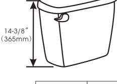
Fixture dimensions and hydraulic performance meet or exceed ANSI/ASME standard A112.19.2M and CAN/CSA B-45 requirements.
